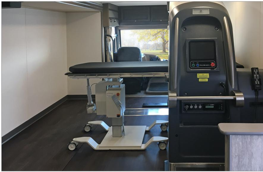
**Approach:** The Mobile CT Clinic features the BodyTom Elite, the world's first portable battery-powered full-body 32-slice CT scanner. A lithium-ion battery-based energy management system replaces the traditional generator to provide on-board power while reducing vehicle emissions.
